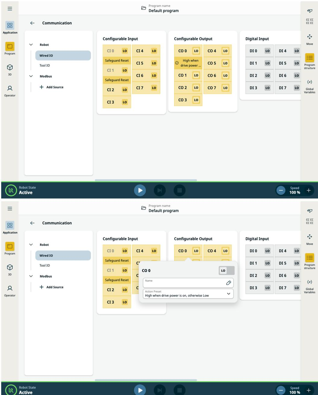
The image displays two screenshots of the Universal Robots software interface, specifically the 'Communication' configuration screen. The top screenshot shows the 'Configurable Output' section with a grid of output buttons (CO 0 to CO 7). The bottom screenshot shows a configuration dialog for 'CO 0' with the action preset 'High when drive power is on, otherwise Low' selected.
